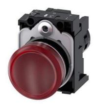
Indicator lights, compact, 22 mm, round, plastic, red, lens, smooth, with holder, Operating voltage 230 V AC, screw terminal
