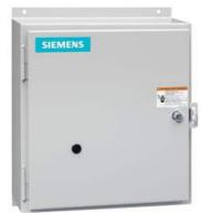
Electrically held lighting contactor, Contactor amp rating 30A, 0 N.C. / 3 N.O. Poles, 220VAC 50HZ/240VAC 60HZ coil, Non-combination type, (no disconnect device), Enclosure NEMA type 12, Dust/drip proof for indoors
