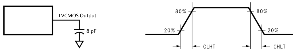
Figure 2. LVCMOS Output Load and Transition Times
