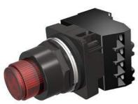
30mm BlackMax, Epoxy Coated Corrosion Resistant Complete Metal Unit PTT / Illuminated Pushbutton Full Voltage, 6V AC/DC Incandescent Lamp Extended Button Plastic Lens, Red 2 Position Momentary with 1 N.O. - 1 N.C. Heavy Duty Contacts, A600/P600 UL Listed, CSA Certified NEMA 1,3,3R,4,4X,12,13 & Automotive Standards
