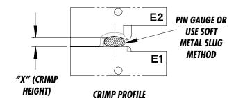
Use gauge pins or soft metal slug (solder) to measure the "X" dimension. Verify tooling crimp
