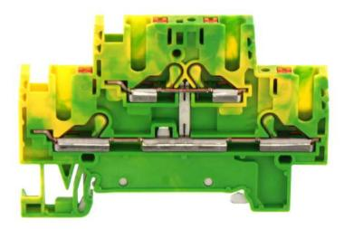
Protective-earth double-level terminal, Push-in connection, Mounting type: Mounting rail TS 35/7.5, Rated cross-section: 2.5 mm<sup>2</sup>, Width: 5.1 mm, Colour: Green-yellow
