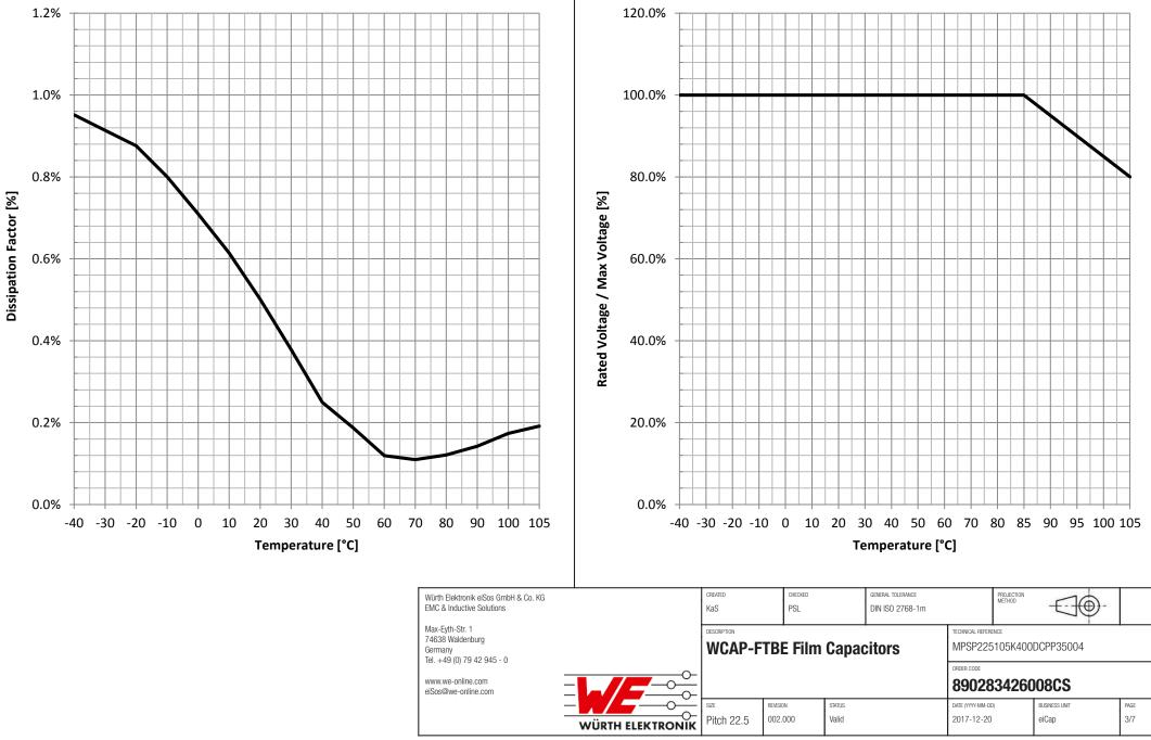
**Rated Voltage vs. Temperature:**
