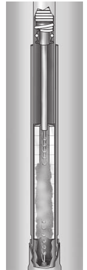
Vapor quenches arc at first current zero
