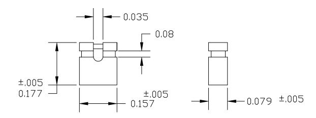
MATERIAL: HOUSING: GLASS FILLED THERMOPLASTIC, UL 94V-0, BLACK
