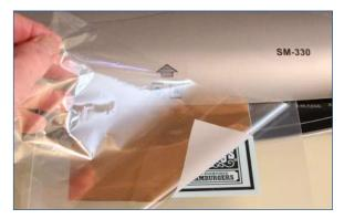
Shown with Carrier Board supporting printed page ovelaid with foil, passing through the laminator.
