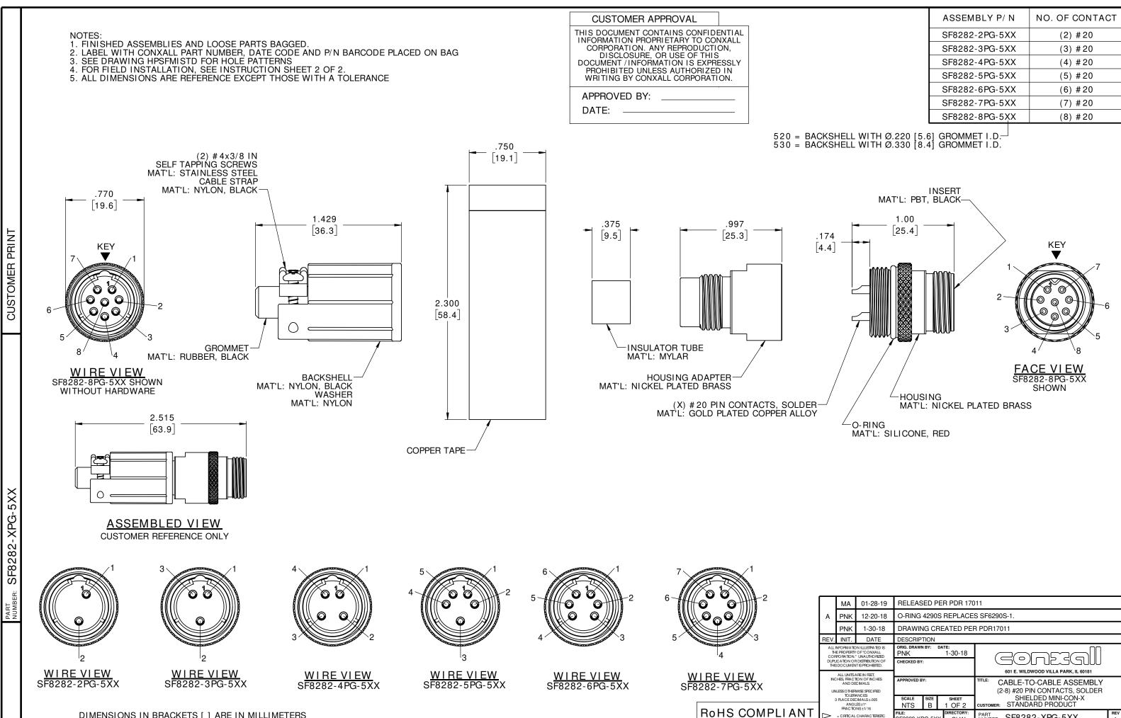
DIMENSIONS IN BRACKETS [] ARE IN MILLIMETERS
