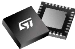
VFQFPN32 exposed pad down (5x5x1 mm)
