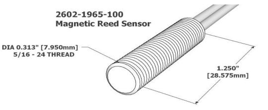
All measurements are in Inches [millimeters]
