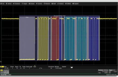
Trigger on exactly the message packets you want with powerful conditional DATA triggering. Apply a color-coded, easy-to-understand, decode over your LIN messages. Search for and find specific message packets in long acquisitions.
