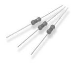
The resistive element comprises a resistive film sputtered onto a ceramic element. Metal end caps are force fitted to the element prior to spiralling. Tinned copper lead wires are welded to the end caps and the components are then coated with four layers of a flame-proof cement. All resistors are tested for value and tolerance. The technology allows the manufacture of custom fusible characteristics.
