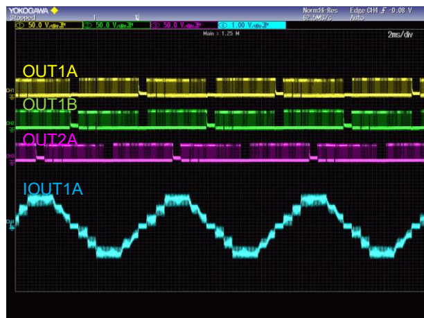
Figure 17. QUARTER STEP ( CLK : 2400Hz )
