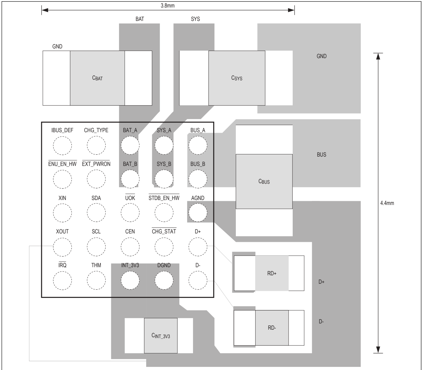
Figure 27. Recommended PCB Layout for Low Speed
