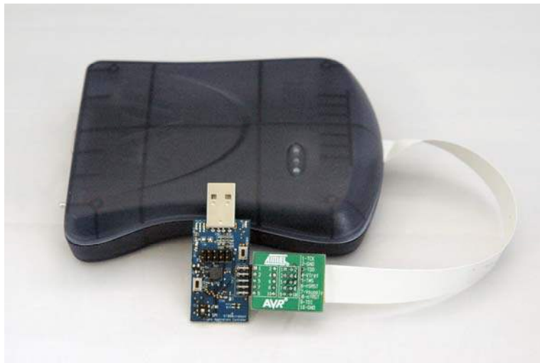
Figure 20. Connecting AVR JTAGICE mkII to the AT88Microbase
