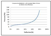
21-869 Gap Pad 1.0mm thick; 1 inch^2 test sample;
