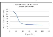
21-869 Gap Pad 1.0mm thick; 1 inch^2 test sample; Pressure step = 10psi
