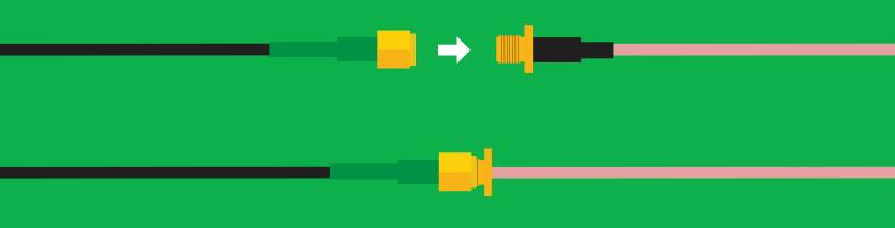
If you need to water proof a SMA connection, we highly recommend using a product like **Coax-Seal** to safely cover and prevent any water damage that may occur.
