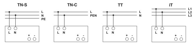
The 100 V AC ... 240 V AC connection is made using the L and N screw connections. The device can be connected to 1-phase AC networks or to two of the phase conductors of three-phase systems (TN, TT or IT networks in acc. with VDE 0100-300/IEC 60364-3) with nominal voltages of 100 V AC ...240 V AC.
