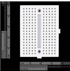
**Description:** This white Mini Breadboard is a great way to prototype your small projects! With 170 tie points there's just enough room to build and test simple circuits; They're also great for breaking out DIP package ICs to jumper wires! If you run out of room, no worries, these mini breadboards can be snapped together to form larger stretches of board. It has a peel and stick adhesive backing as well as two mounting holes for M2 screws so you can anchor it down.
