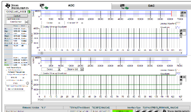
Figure 189. Idle-Channel Noise (No Input) for 2.5-GSPS, Dual-Channel Oscilloscope
