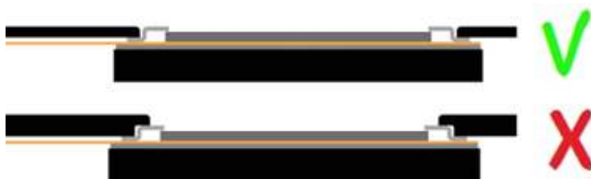
Figure 19. Positioning of the sensor
