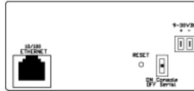
IOLAN SDS1 TA4D2 – 4 Analog inputs and 2 Digital I/O and 1 RS-232/422/485 Serial Port
