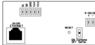
IOLAN SDS1 TA4D2 – 4 Analog inputs and 2 Digital I/O and 1 RS-232/422/485 Serial Port
