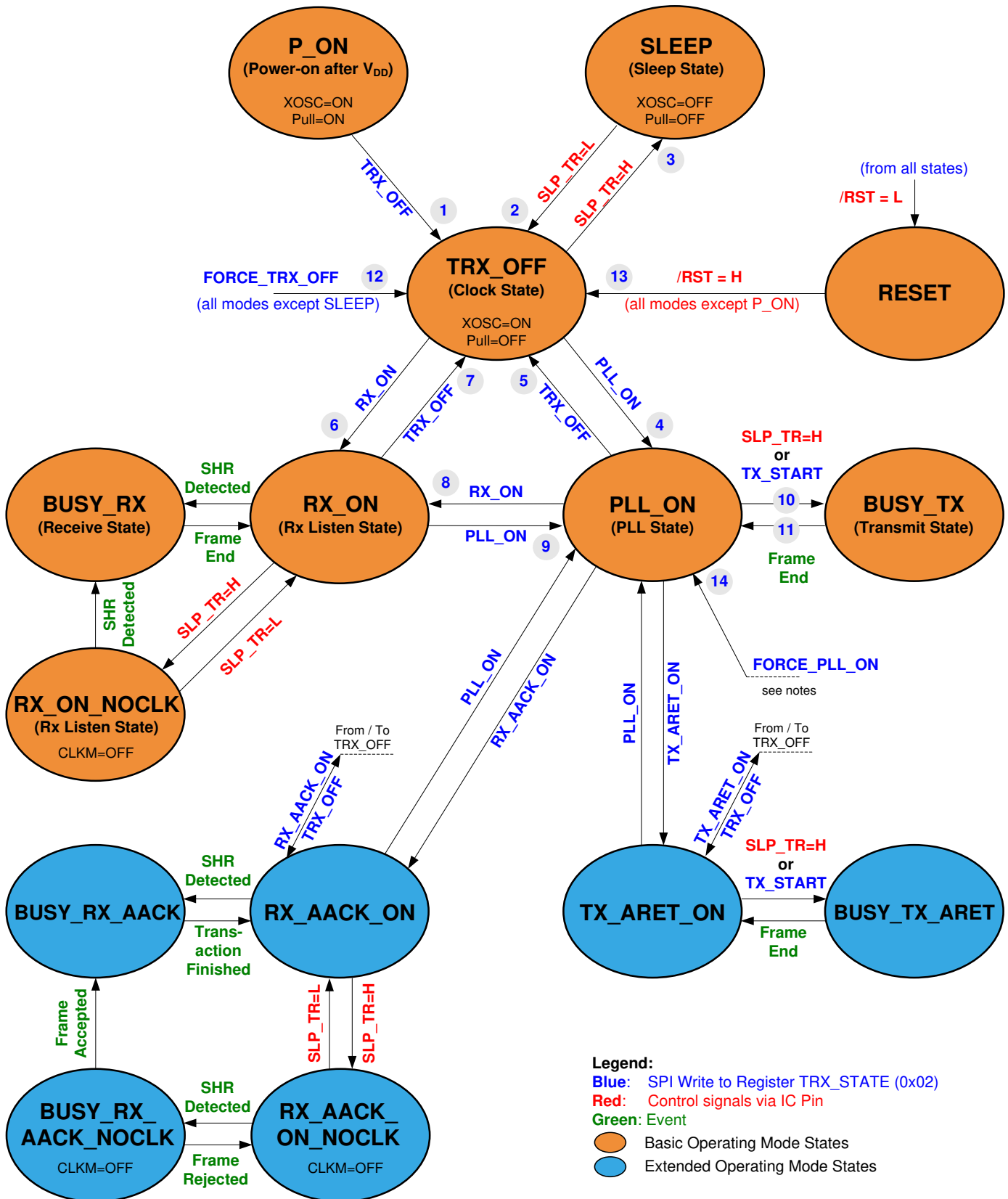
Figure 7-10. Extended Operating Mode State Diagram.
