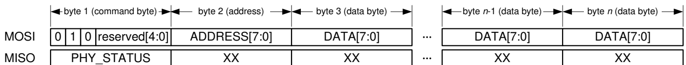
Figure 6-12. Packet Structure – SRAM Write Access.
