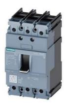
circuit breaker 3VA5 UL frame 125 breaking capacity class S 25kA @ 480 V 3-pole, line protection TM210, FTFM, In=70A overload protection Ir=70A fixed short-circuit protection Ii=10 x In UL489 SB (naval), 50 deg. cel. cable connection on both sides
