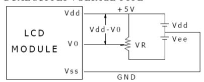
Vdd-V0: LCD Driving Voltage
