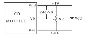
Vdd-V0: LCD Driving Voltage
