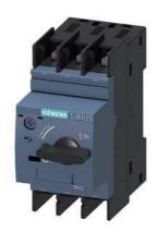
Circuit breaker size S00 for motor protection, CLASS 10 A-release 0.55...0.8 A N-release 10 A ring cable lug connection Standard switching capacity
