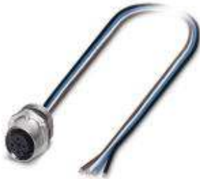
Sensor/actuator flush-type socket, 4-pos., M12 SPEEDCON, A-coded, front/screw mounting with M16 thread, with 0.5 m TPE litz wire, 4 x 0.34 mm 2
