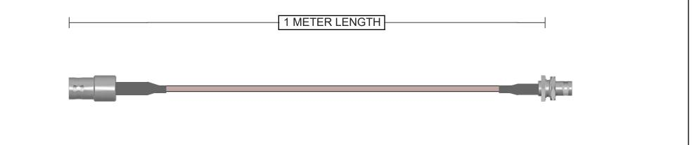
Connector A 112161 BNC Jack Straight Brass Nickel + Heatshrink 75 Ohm RG-179 Continuity/Hi-Pot Connector B 112235 BNC Jack Straight Bulkhead - Rear Mount Brass Nickel + Heatshrink
