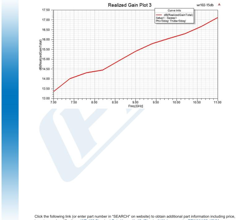
inventory and certifications: WR-102 Standard Gain Horn with 15 dBi gain, N Male connector PEWAN102-15NM
