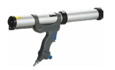
Pneumatic gun has a 10.3 oz. cartridge dispenser that also works for 10 oz. sausage cartridges. It has a series 3 air action system, piston rod action cartridge plunger or sausage, 145 psi max input, and a drawn aluminum barrel.
