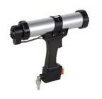
Pneumatic gun with a 10 oz. cartridge dispenser. It has air action cartridge plunger, 145 psi max input, and a drawn aluminum barrel. With a true adjustable air regulator, this can output up to 75 psi. Includes a rotating air hose connector.
