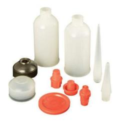
Cartridges are an alternative product when syringes have too small of a capacity. Cartridges are available in low or high density and offered in three different capacities (2.5oz., 6oz. and 12oz.). Cartridge accessories include plunger wipers, end caps and threaded plugs. 1/4" threaded nozzles screw into the cartridge for bead and dot dispensing. Dispensing nozzles are used in conjunction with cartridges when the application requires a reservoir larger than a syringe.
