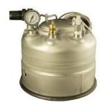
These tanks allow for material storage and dispensing. Each tank comes with a regulator, gauge and pressure relief valve. They are available in 1, 2, 3 and 5 gallon capacities.
