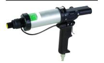
Two-part epoxy pneumatic gun that accepts a 1:1 ratio dual syringe cartridge (usually bought pre-filled from a material manufacturer). Dual syringe is a  $25 \times 25$ ml syringe of material.
