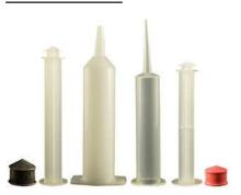
Our one-piece molded barrels are made of polypropylene and do not require a dispensing tip to operate. This natural colored syringe is available in four different tip sizes and offer a great alternative for dispensing thicker materials. The tapered tip can be cut back to widen the opening and allow more material to flow. The JG30MT (using the JG30T-1N barrel) has a tip ID of .0385"; the JG30MTL (using the JG30T-1L barrel) has a tip ID of .170".
