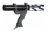
Dual pneumatic gun with a 200 ml capacity for various two part applications. The ratio has several different variations, of 1:1, 2:1, 4:1 and 10:1 with the kits included. It has a twist and lock plunger feature to easily switch between ratios. This unit has an adjustable air regulator at 100 psi and the maximum output of this gun is 145 psi. Nominal thrust 484 lbs.
