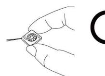
Don't pull fan with lead wires.
