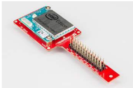
Headers on Edison side
