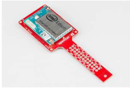
Edison installed on Pi Block
