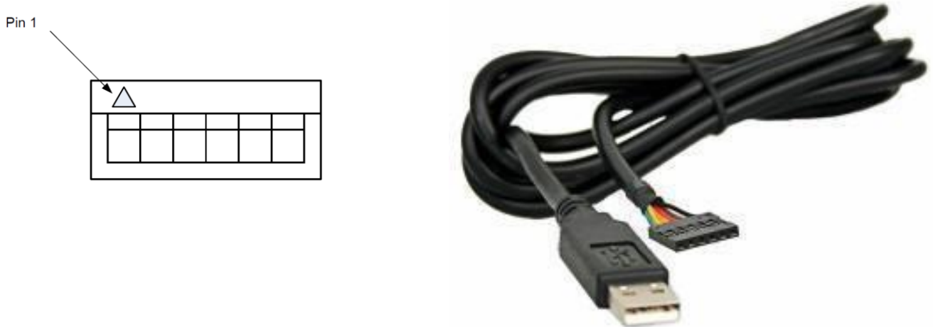
FIGURE 6 - PIN HEADER SOCKET BOTTOM VIEW
