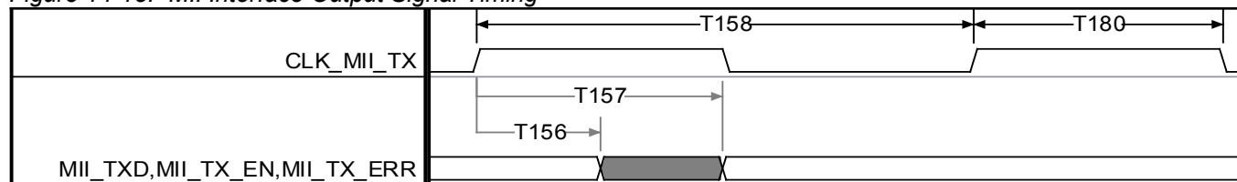
Figure 14-15. MII Interface Output Signal Timing
