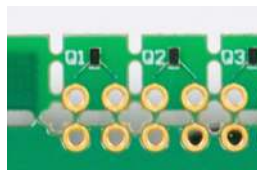
Figure 8. Remote Junction Transistors
