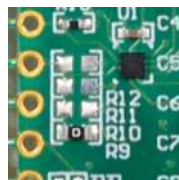
Figure 7. EVM Address Pin Hole Connections
