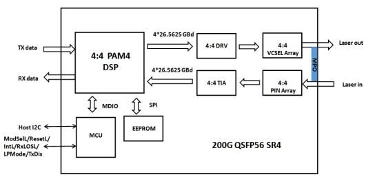
*Transmitter Section:* This module converts 4-channel 53.125Gbps electrical data to 4-channel 850nm 53.125Gbps optical signals for 212Gbps optical transmission.
