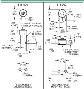
For dimensions  $\leq$  .125"/3.18mm, tolerance is  $\pm$ .005/0.13 For dimensions  $\geq$  .126"/3.20mm, tolerance is  $\pm$ .015/0.38
