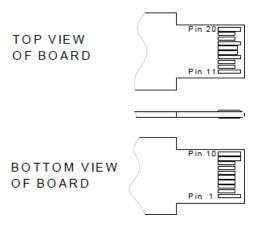
Pin-out of connector Block on Host board
