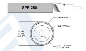
SPF-250 Coax Using Times Microwave Parts PE3C6350-60
