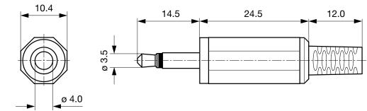
Cable diameter max. 4.0 mm
