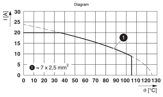
I = current strength,  $\vartheta$  = ambient temperature, 7x 20 A
