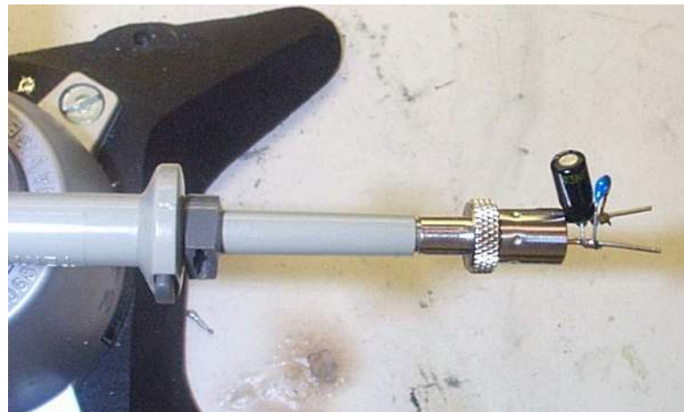
Figure 24 – Oscilloscope Probe with Probe Master ( www.probemaster.com ) 4987A BNC Adapter. (Modified with wires for ripple measurement, and two parallel decoupling capacitors added)
