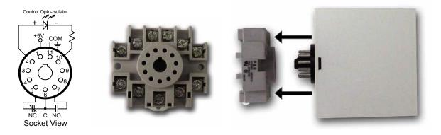
11-pin connector pinout:
