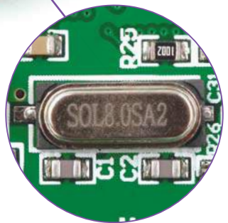
Figure 5-1: External crystal oscillator (X1)
