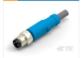
TE Part # T4051120003-002 M8 CABLE ST MALE 1.0M 3P PUR CABLE
