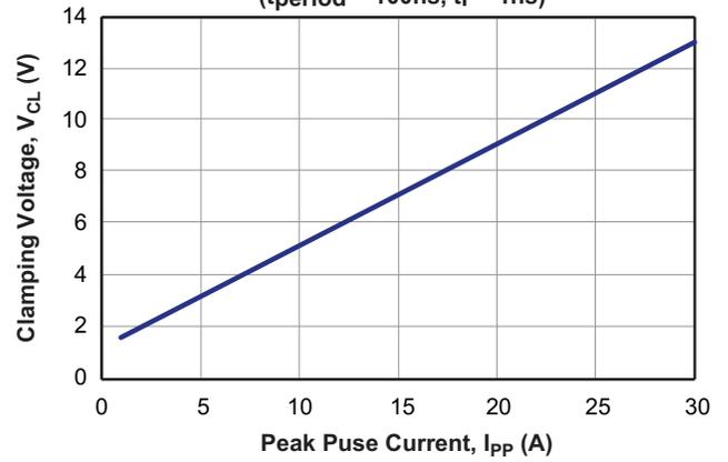
+8kV ESD Clamping Per IEC 61000-4-2
