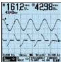
Dual-input measurement shows both meter reading and waveform at the same time (124, incl. cursors)
